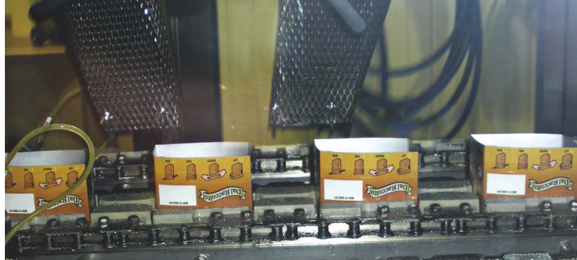
The intermittent-motion form/fill machine handles two cartons simultaneously. Dry components discharge through funnels into the cartons, top photo. Carton blanks are pushed up onto mandrels for forming.
