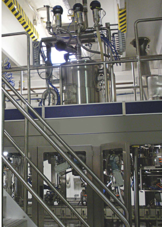
Liquid component is filled from a holding tank on top of the form/fill machine into the cartons by piston fillers.
