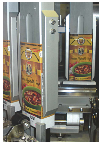
The intermittent-motion form/fill machine handles two cartons simultaneously. Dry components discharge through funnels into the cartons, top photo. Carton blanks are pushed up onto mandrels for forming.
